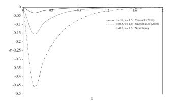
Fig. 8 Dependence of stress distribution on the derivative and integral fractional orders  $\alpha$  and  $\nu$  for different theories.
