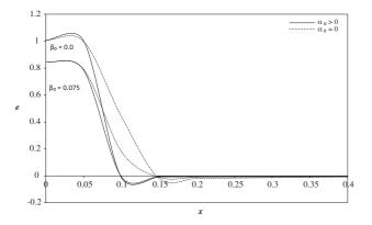
Fig. 7 Dependence of strain distribution on Alfven velocity and temperature discrepancy.
