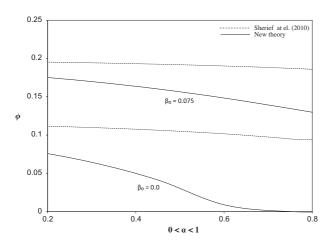
Fig. 2 The conductive temperature distribution against the derivative fractional order  $\alpha$  for different theories.
