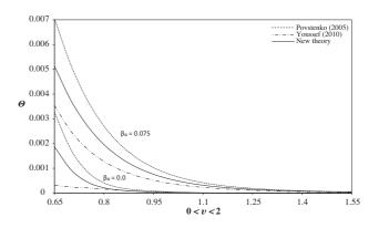
Fig. 3 Dependence of thermodynamic temperature on the integral fractional order v for different theories.
