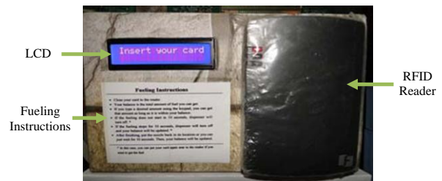
Figure 8. RFID reader and the hardware module enclosure
