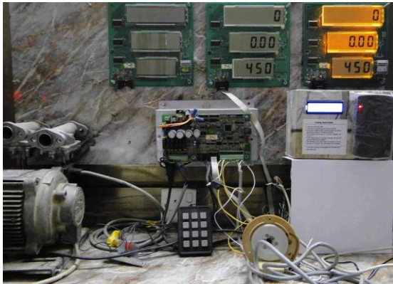
Figure 9. The hardware module connected to dispenser
