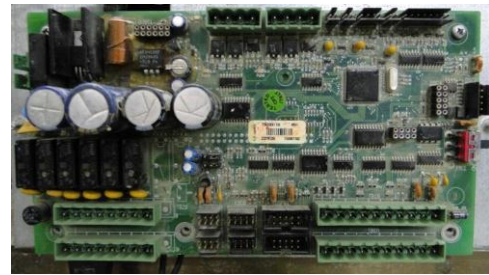
Figure 2. Fuel dispenser embedded system
