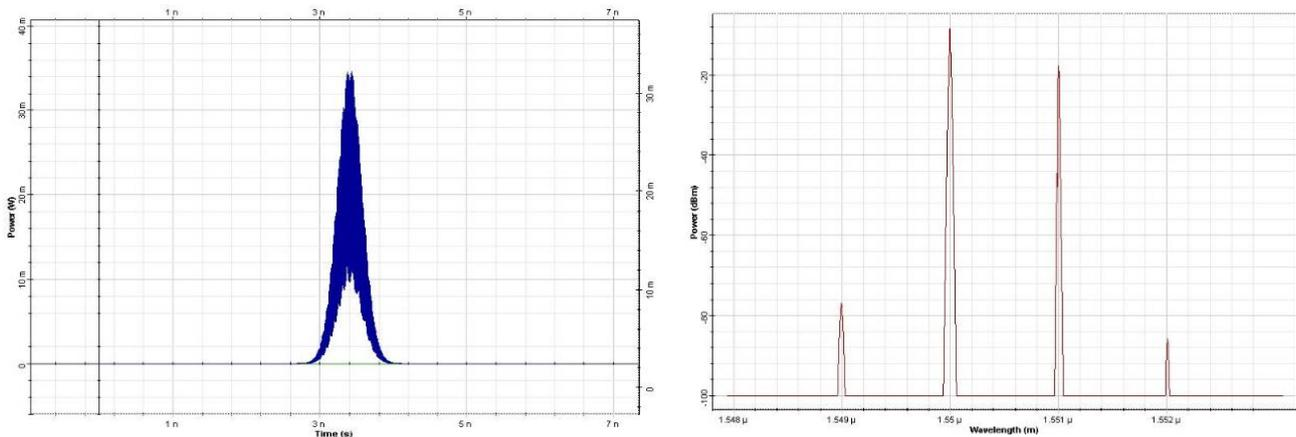
Figure 4. The transmitted pulse and its spectrum for 60 Km transmission distance
