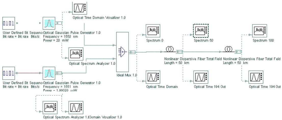
Figure 2. Optical fiber communication project design
