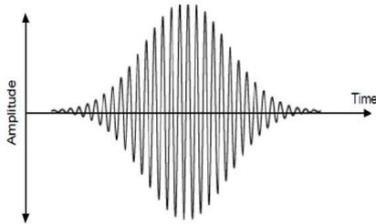
Figure 1(a). The Gaussian pulse (un-chirped)
