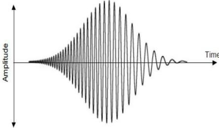
Figure 1(b). The Gaussian pulse (chirped)
