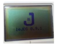
Fig. 7. LeJOS firmware in NXT brick screen.
