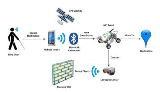
Fig. 1. The system's Block Diagram.
