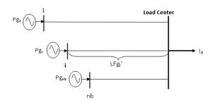
Figure 1. Loss Factor of Bus Generation reffered to Load Center
