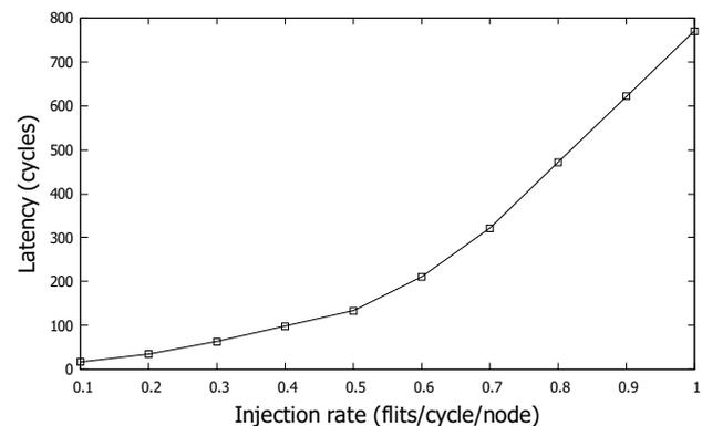
Figure 4. Latency measurements for simulation of  $2 \times 2$  cluster of 4  $2 \times 2$  NoC-based systems.
