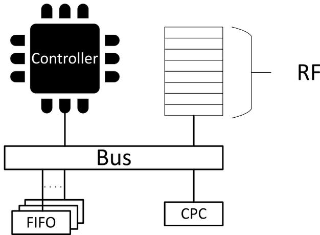
Figure 6. ICFIFO internal structure in NoC<sup>2</sup>.
