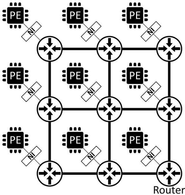
Figure 1. Standard NoC components.
