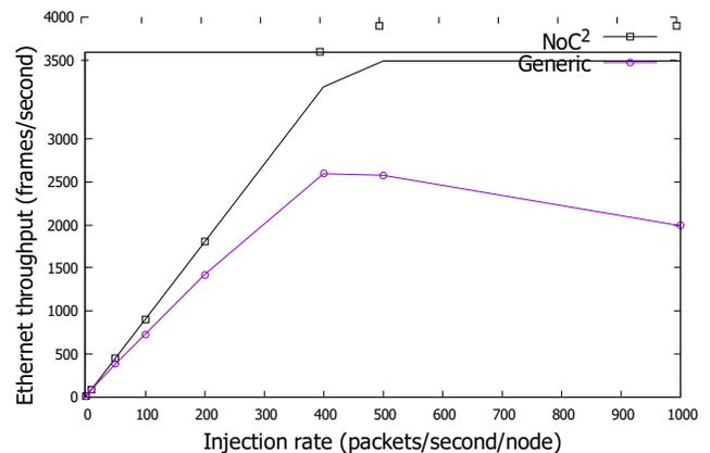
Figure 12. Inter-NoC packet throughput versus PIR.
