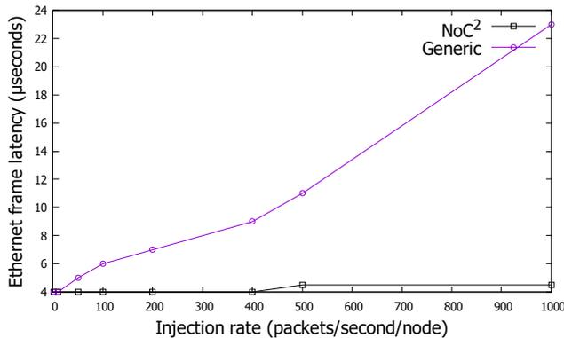
Figure 13. Inter-NoC packet latency versus PIR.
