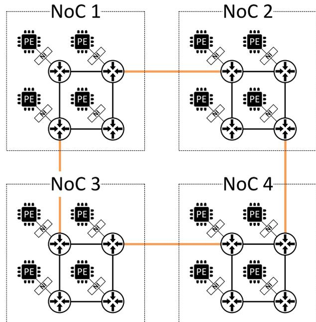
Figure 3.  $2 \times 2$  cluster of 4  $2 \times 2$  NoC-based systems.
