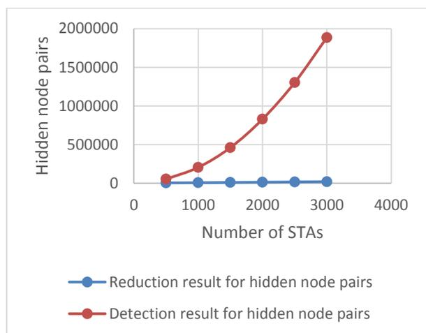
Figure 6: Performance Evaluation for Hidden node pairs
