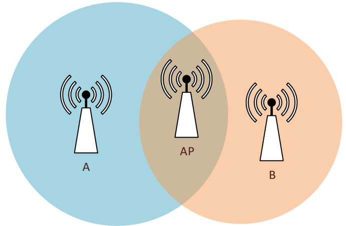
Figure 2: Hidden nodes Node c is hidden from node A and vice versa
