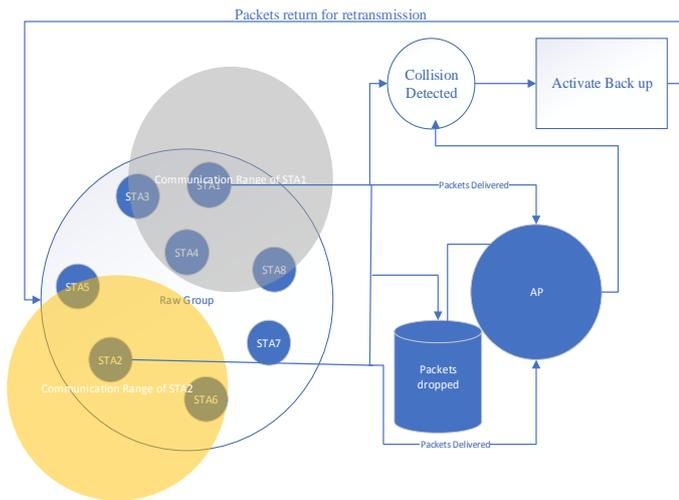
Figure 4: Packet transmission in BIHD-CM
