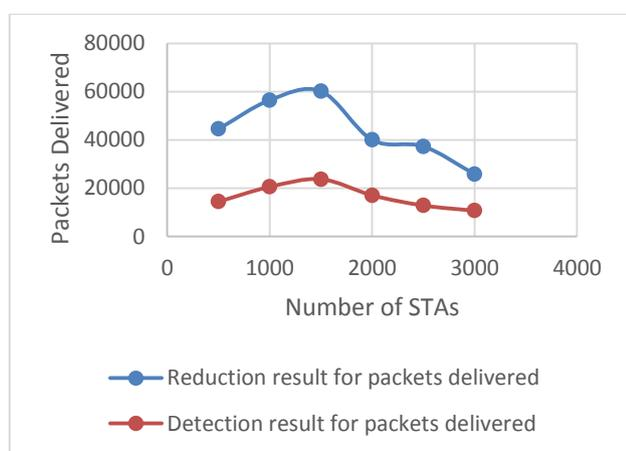
Figure 7: Performance Evaluation for packets delivered
