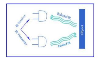
Figure 2: Infrared Sensor Functionality
