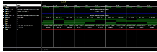
Figure 10. Simulation output waveform of NFSRs updating phase for Basic version of Lizard
