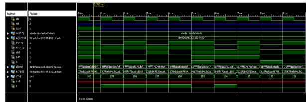
Figure 4. Simulation output waveform of initialization phase for Basic version of Grain v1
