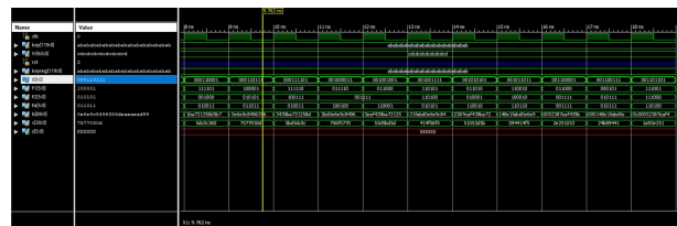
Figure 12. Simulation output waveform of NFSRs updating phase for Parallel version of Lizard
