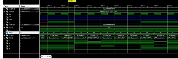
Figure 18. Simulation output waveform of key generation phase for Basic version of Plantlet
