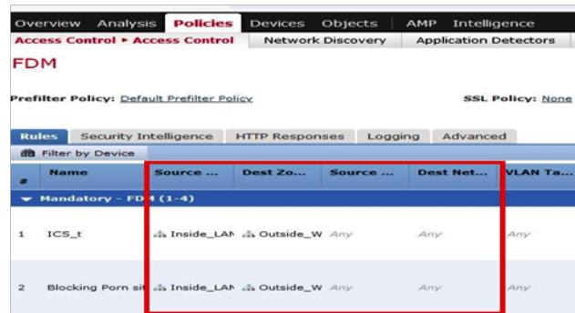
Figure 3. Segmentation using NGFW Firewall at AERE
