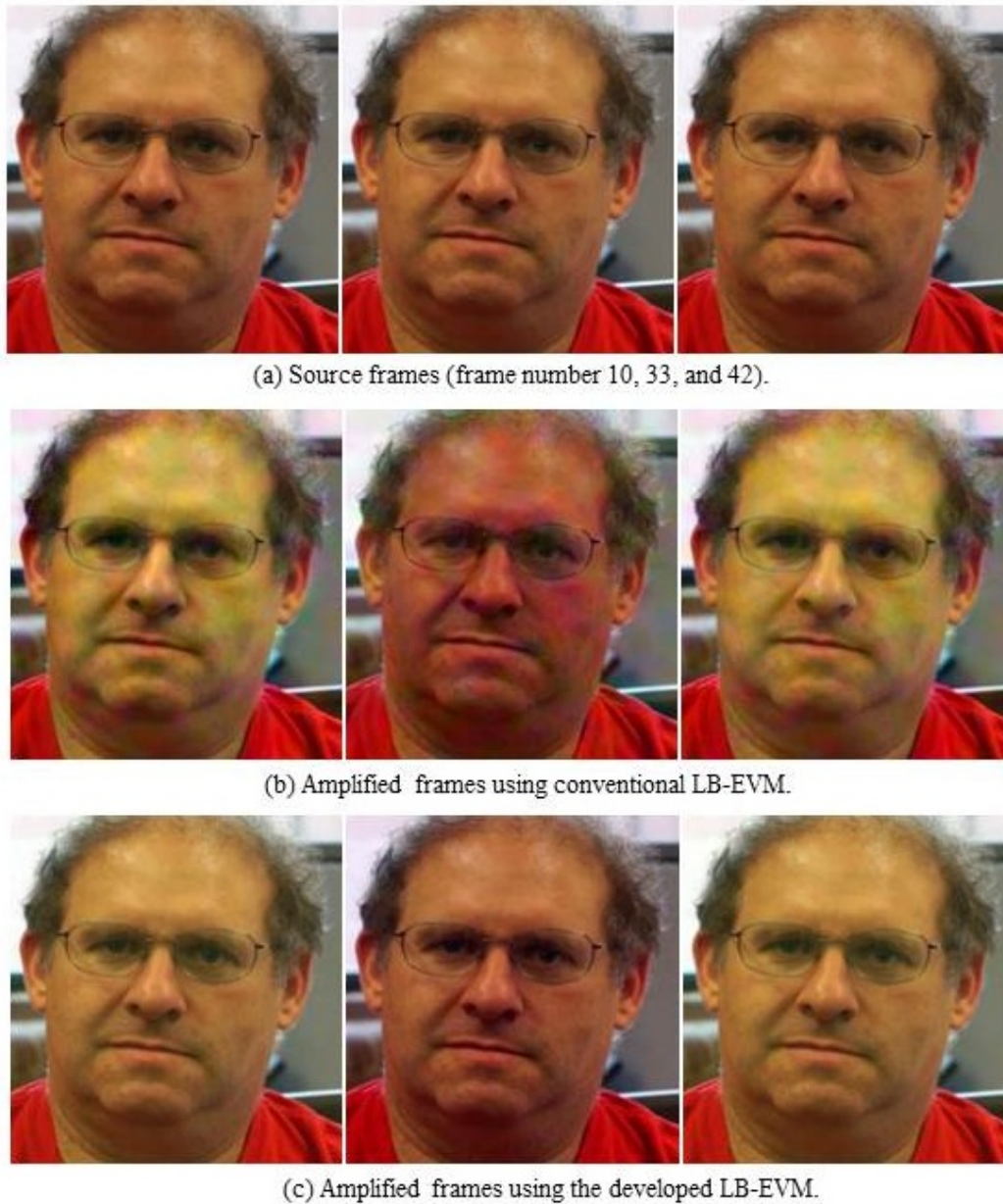
Figure 11. Samples of Face video before and after magnification using conventional and developed LB-EVM approaches at \alpha=200 .
