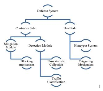
Figure 1. Defense System Modules Diagram.
