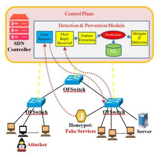
Figure 2. The Framework of The Proposed Mechanism.
