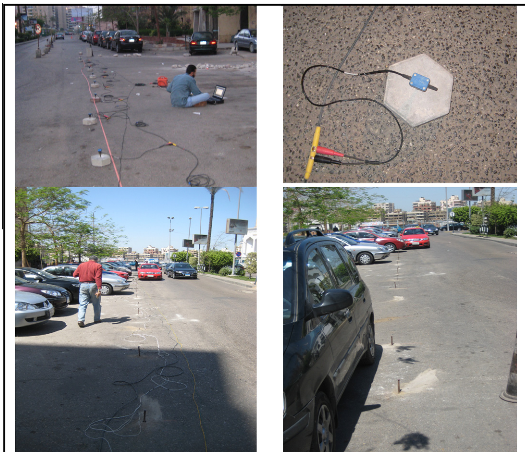
Figure 5 Acquisition processes of the MASW data using geophones attached to concrete plates and the ERT data where long steel electrodes were used to penetrate the asphalt down to the conductive soil layer underneath the asphalt.
