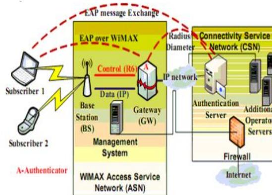
Figure 4. Authentication Based on EAP [2]
