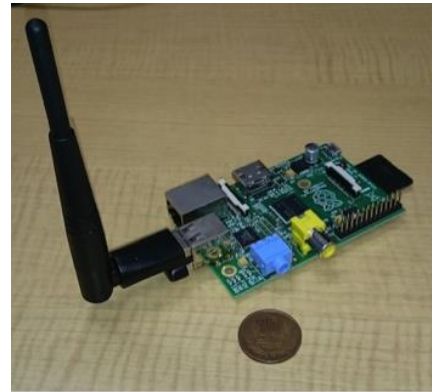
Figure 5. Wi-Fi beacon emitter
