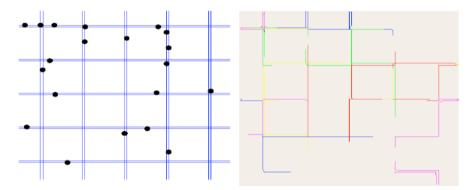
**Figure 2.** Plots of (left) 20 nodes randomly distributed by MG model and (right) footprints of nodes Maximum velocity: 2m s-1, grid size: 500x500m, simulation time: 250 sec, zero pause time (continuous motion)
