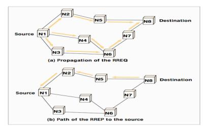
Figure 1. AODV route discovery process (from [14])
