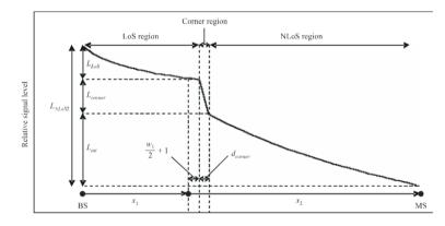
**Figure 3.** Typical trend of propagation along street canyons with low base station height for frequency range from 2 to 16 GHz (from [21]).
