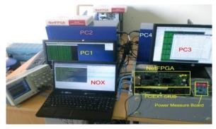
Figure 11. The experimental setup with NetFPGA switch, an extender board, NOX controller and host PCs
