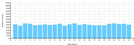
Figure 4. Number of events per hour generated by a temperature sensor. Standard deviation is below 150. This indicates a sensor not monitoring human behaviour.
