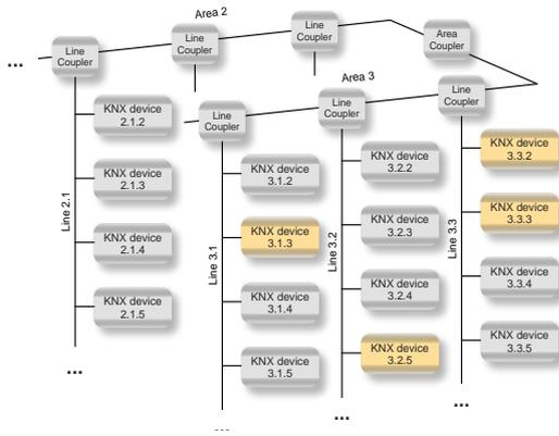
Figure 2. Example for the structure of a KNX network showing two areas with several lines and several devices per line.
