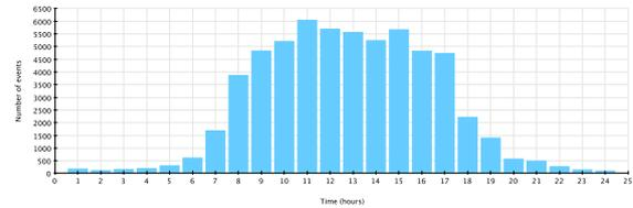
Figure 5. Number of events per hour generated by a temperature sensor. Standard deviation is below 150. This indicates a sensor not monitoring human behaviour.
