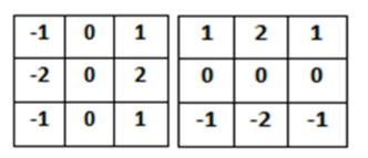
Figure 3. Sobel Masks for edge detection
