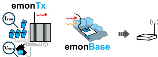
Figure 9. Hardware Architecture of the iTrack Prototype
