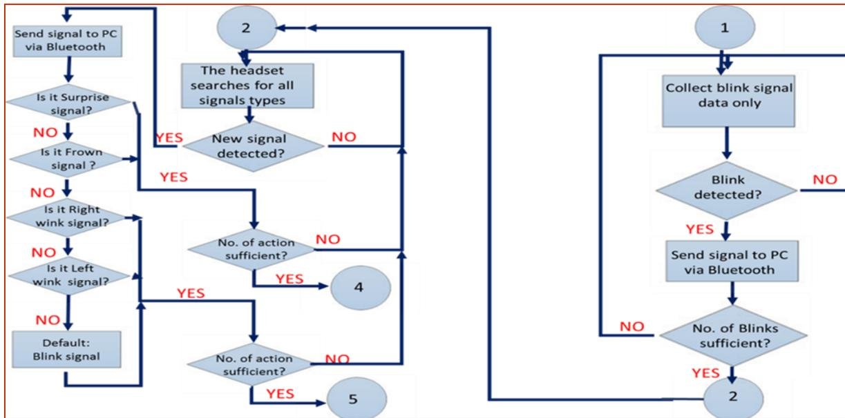
Figure. 2b. Signal processing in PC.
