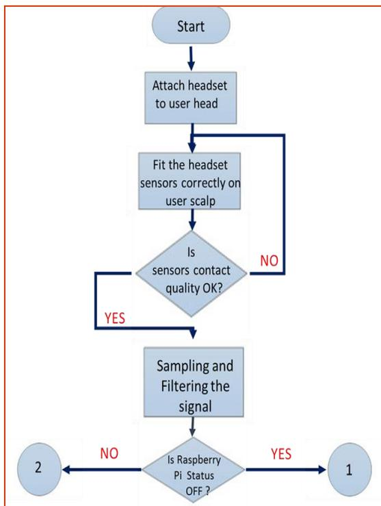
Figure 2a. Headset connection flowchart.
