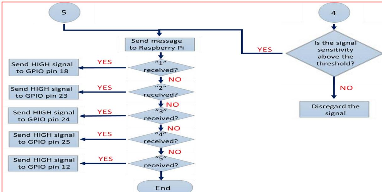
Figure. 2c. Signal processing in Raspberry Pi
