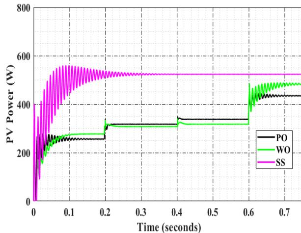
Figure 8. Characteristics of PV array - PV output power for three MPPT techniques.
