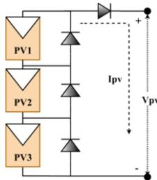
Figure 3. 3S PV array configuration.
