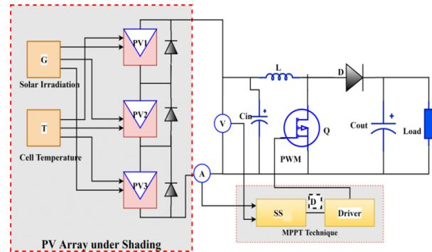
Figure 6. Block diagram of the proposed SS MPPT technique.
