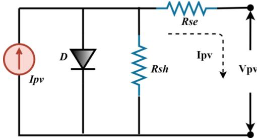
Figure 1. Equivalent circuit of the PV cell.
