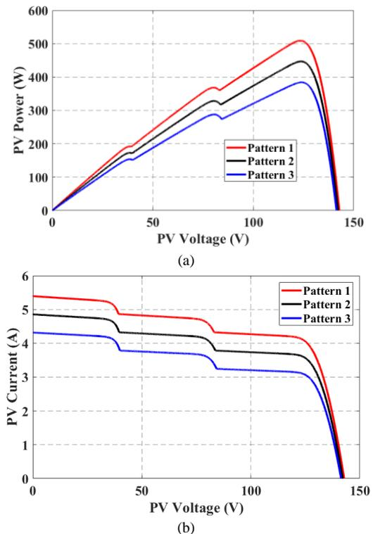
Figure 2. PV panel characteristics under PSCs; (a) P-V characteristics, (b) V-I characteristics.
