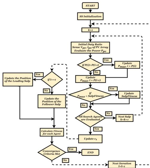
Figure 5. Overall flowchart of the proposed SS MPPT method.
