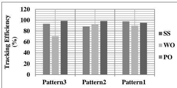
Figure 11. Tracking efficiency of various MPPT techniques
