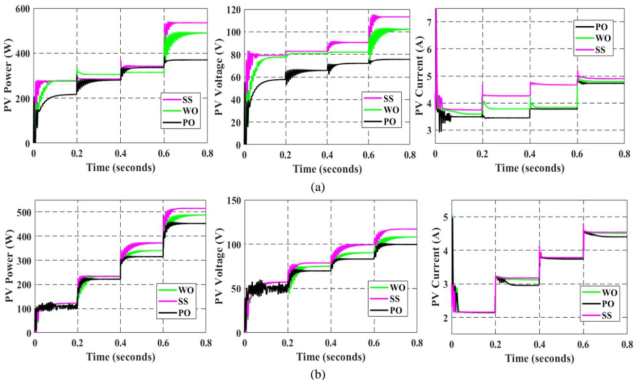
Figure 9. Tracking characteristics; (a) Rapid change in insolation, (b) Extreme change in insolation.
