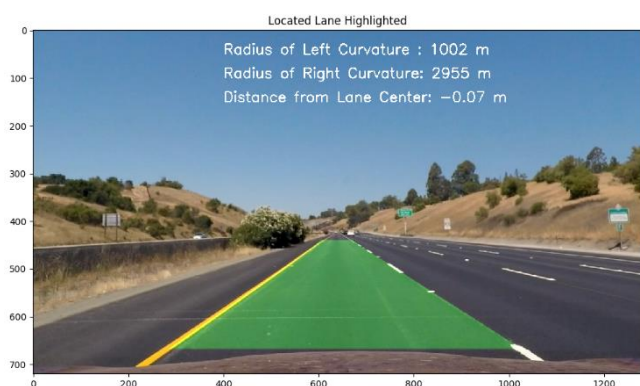
Figure 18. Identified lane lines highlighted in green and the measured lane curvatures.
