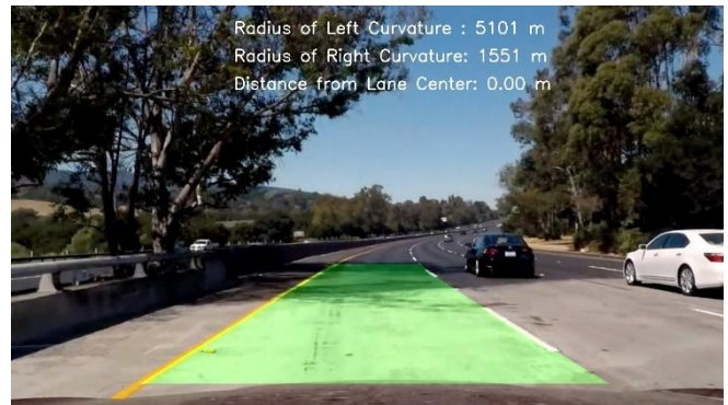
Figure 23. Test image with solid yellow and dotted white lane lines segments (left turning lane with scattered shadows, and cars).
