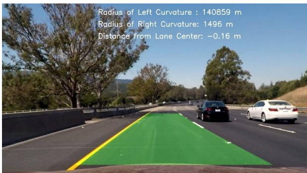
Figure 1. Detected lane boundaries by the LaneBD algorithm.
