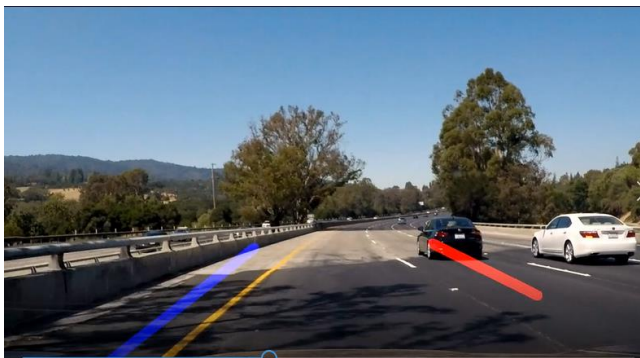
Figure 25. Test image with solid yellow and dotted white lane lines segments (left turning lane with scattered shadows, and cars) using LaneRTD [43].
