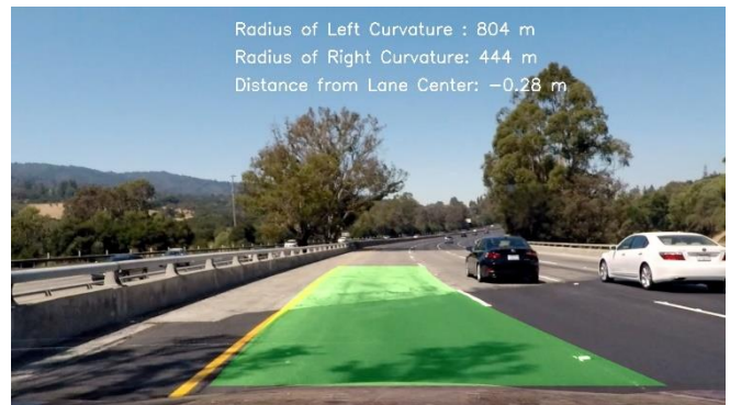
Figure 22. Test image with solid yellow and dotted white lane lines segments (left turning lane with scattered shadows, and cars) using LaneBD .
