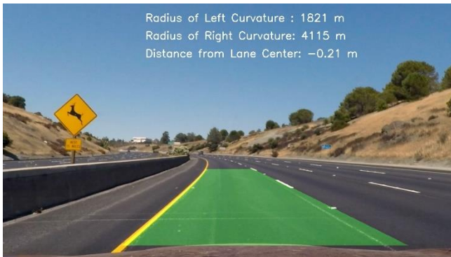
Figure 20. Test image with solid yellow and dotted white lane lines segments (road at sunset (dusk), left lane with no cars).
