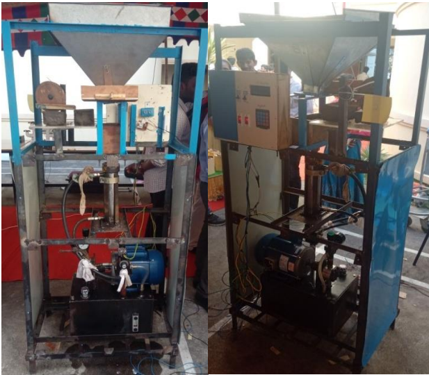
Figure 6. Working prototype of smart and integrated brick making machine
