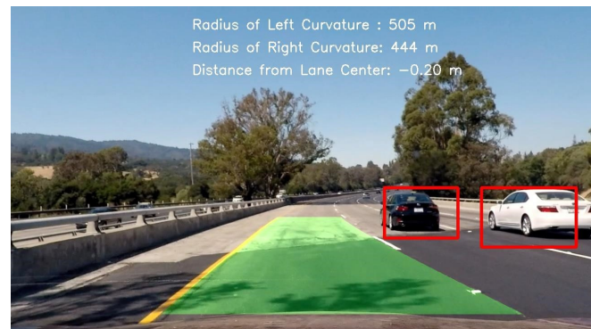
Figure 2. Detected Vehicles’ boundaries by the RT_VDT algorithm.
