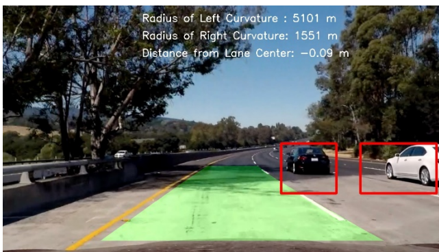
Figure 19. The execution of vehicle detection and tracking pipeline.
