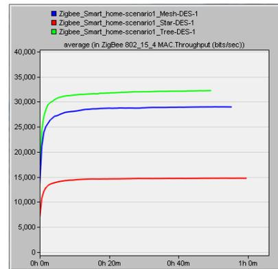
Figure 8. Average throughput for 1ZC ZigBee network in global mode
