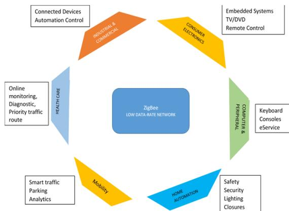
Figure 4. ZigBee Applications
