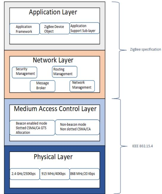
Figure 2. ZigBee Layers
