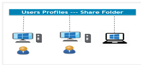
Figure 4. Users Files and Profiles are Stored in Data Center and Can be Accessed from Any Device
