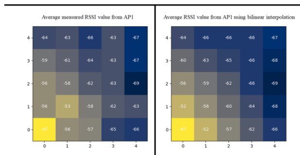
Figure 21. Comparison of the mean RSSI value of measurement results and Neville interpolation
