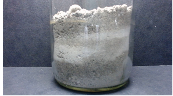
Figure 4. Soil Mixture After-Process – After Settling
