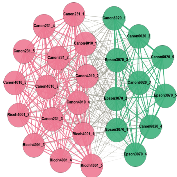
Figure 8. Group 5: Visualization of ink spectrums of five printers. The network is separated printers into two clusters. The first includes inks for laser printers and the second includes inks for inkjet printers.
