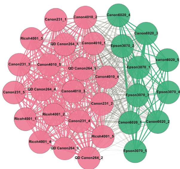
Figure 9. Group 6 Test 1: Visualization of the questioned document's spectrums that was printed using the laser printer (Canon 264). The spectrums were clustered with the cluster of the same type of printing.
