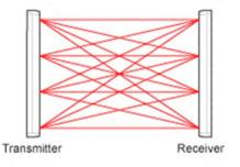
Figure 2. Sending and receiving IR beams
