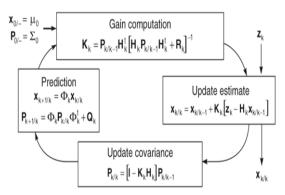
Figure 1. Operation of Kalman filter
