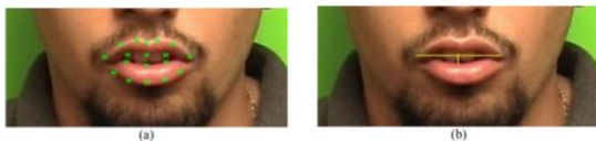
Fig. 7: (a) landmarks of the lips (b) width and height as lips feature [36].
