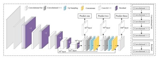
Figure 1. YOLOV3 network architecture [43]
