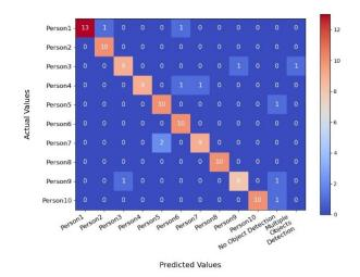
Figure 15. Matrix of MobileNet-SSDV2 Test Result
