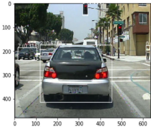
Figure 3. Qualitative results of the pre-trained Tiny-YOLOv3 model on the Caltech Pedestrian dataset (detect 80 object categories)
