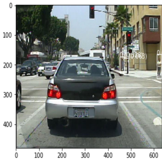
Figure 4. Qualitative results of the fine-tuned Tiny-YOLOv3 model on the Caltech Pedestrian dataset (detect only pedestrian object)
