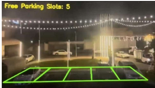
Fig. 6. Fail in detecting vehicles during evening
