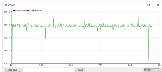
Figure 3. The collection of the sensor values in serial monitor
