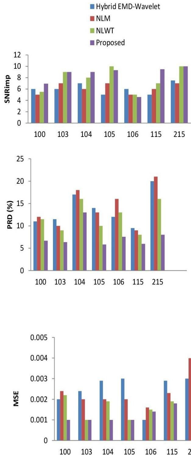
Figure 9. Denoising Performance Proposed Algorithm on different Records from MIT-BIH Database at 20 dB SNR
