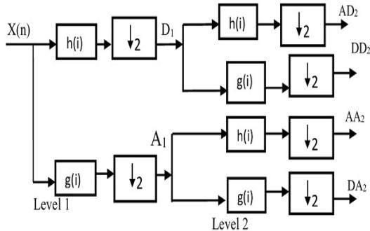
Figure 3. Two level decomposition, using WPT
