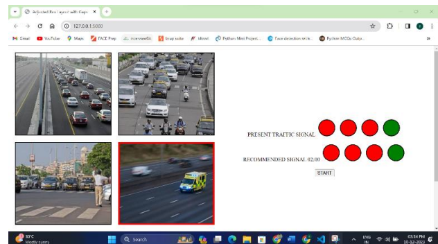
Figure 5: Interface showing Ambulance detected CCTV box along with recommended signal
