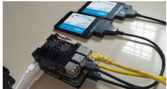
Figure 3. Edge Cluster power usage is typically around 45W at peak processing demand
