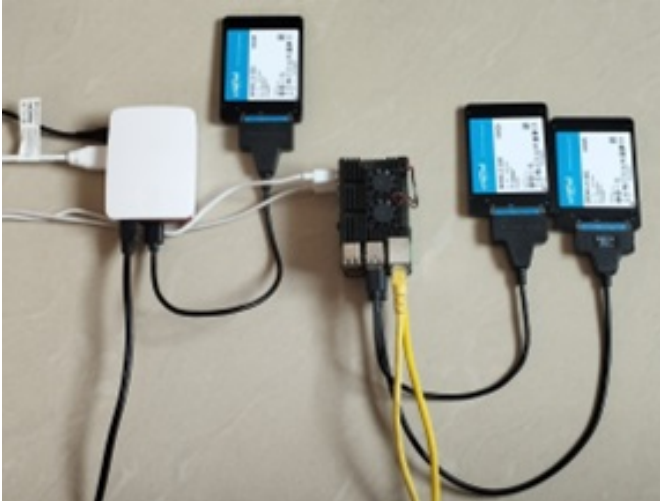
Figure 1. SBC cluster connections with two RPi 4 – 8GB and one RPi 3B+ Storage Controller
