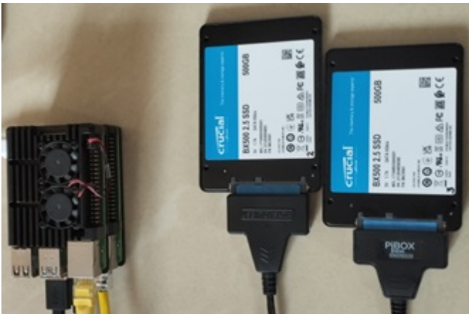
Figure 2. USB SSDs ensure quick bootup and optimal edge performance with 300Mb/s throughput
