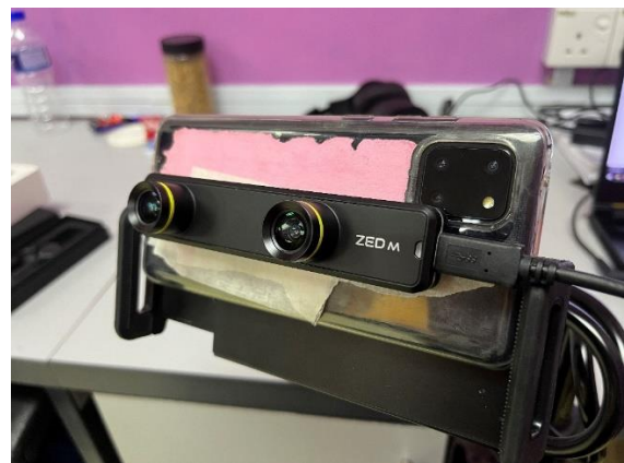
Figure 2. Attachment of ZED Mini to handheld device
