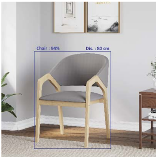
Figure 6. Drawing Bounding box with Class name, and prediction confidence, and distance.
