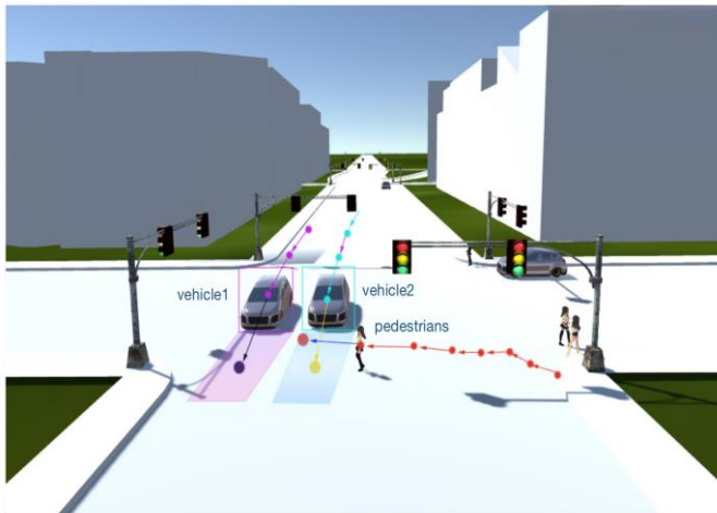
Figure 3. A Computer Vision-Based Algorithm for Detecting Vehicle Yielding to Pedestrians [33].
