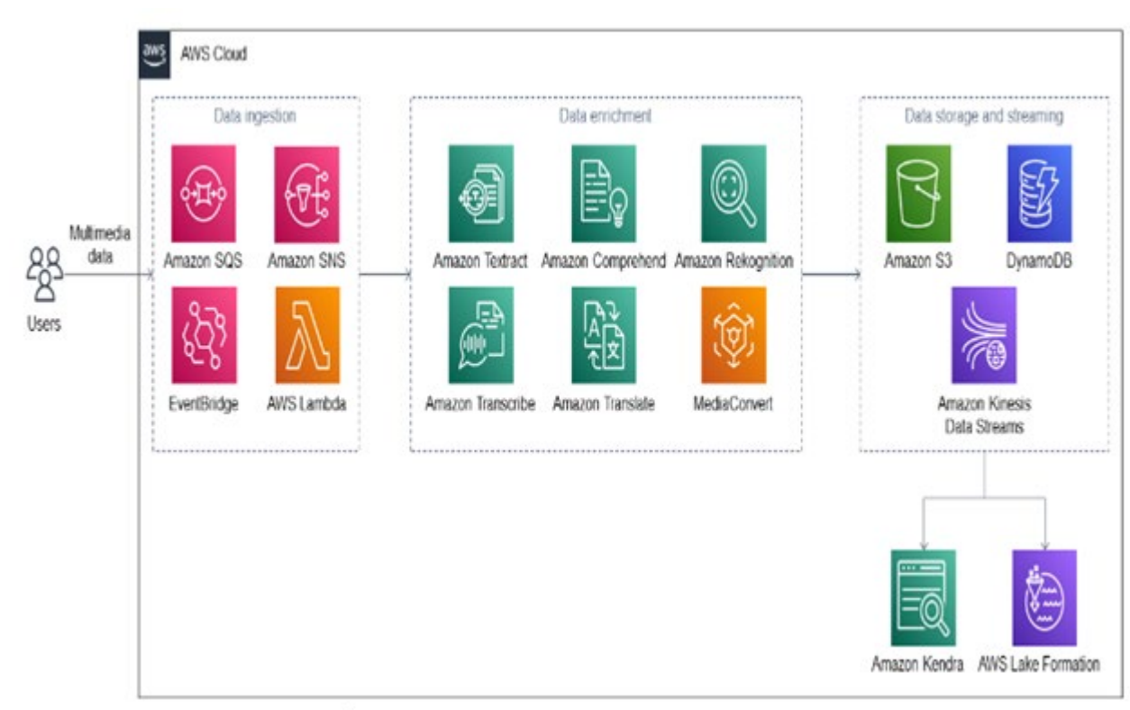
[9] Figure 3: AWS Architecture
