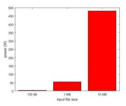
Figure 13: Device power saved by offloading to the cloud for different file sizes
