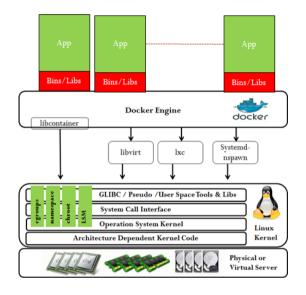
Figure 3: Containerization of Mobile Applications
