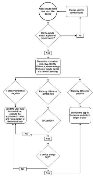
Figure 2: Flow diagram of implemented algorithm
