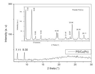
Figure 3 X-ray diffraction patterns of Cu-Pc/PS thin films.
