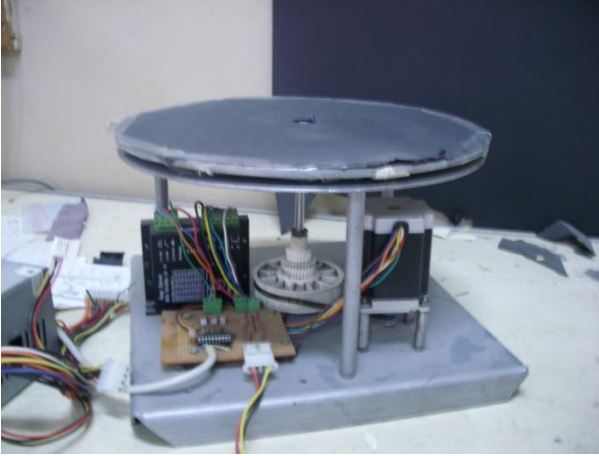
Figure 1. The rotary table is used in our work to change the camera's viewing direction to an object.
