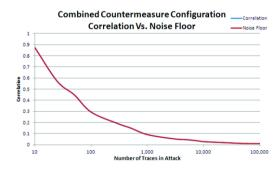
Figure 9. Combined Countermeasure - Correlation Vs. NoiseFloor-100K Traces
