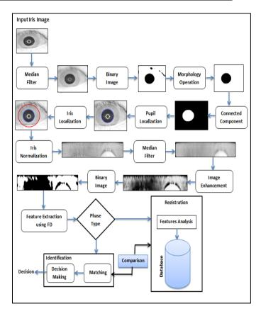
Figure 6. The proposed system procedure.
