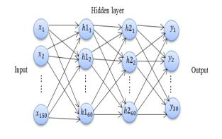
Figure 5. Architecture for BP neural network
