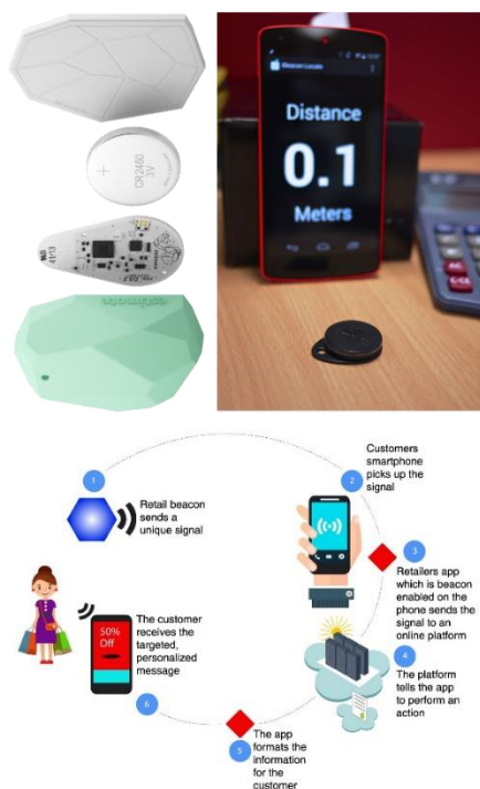
Figure 8. Bluetooth low energy Beacon and its application scenario (photo: google).
