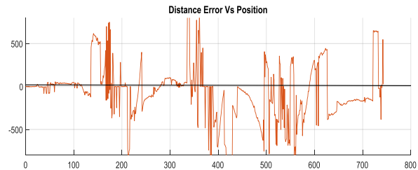
Figure 7: experimental cross track error result of scaled vehicle following the desired reference
